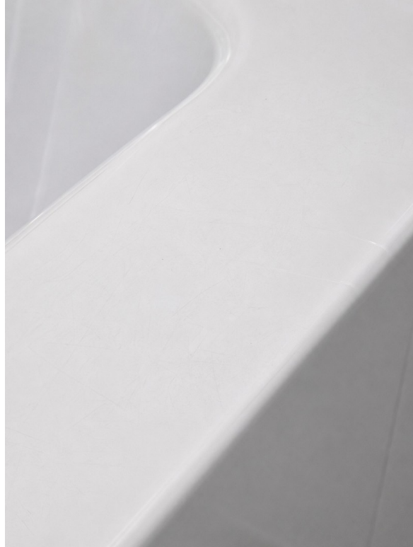
Close-up example of scratching on a smooth acrylic surface.
